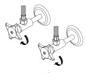
1. Shut off water supply. Remove old faucet. Clean mounting surface in preparation for new faucet.
