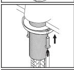
(2c) Thread locknut onto the faucet shank from underneath the sink. Position faucet to desired location from the top and handtighten locknut till it won't go further. Thread both screws on locknut and tighten screws on locknut with the help of a Phillips head screwdriver to secure faucet. (Note: Do not
