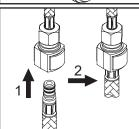
(5) Insert spray head hose into end of quick connect adapter on the outlet hose, push until a "click" is heard. Pull down to test engagement.
