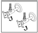
(6) Connect hot and cold inlet supply hoses to supply stops. For supply stop with 1/2" outlet connection, use 3/8" male to 1/2" female adapter for installation. Adapters are optional and are not provided with the faucet. Turn on both side supply stops to check any leaks.
